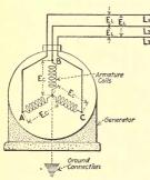
Fig. 237.—Diagrammatic representation of a star- or Y-connected, three-phase generator.
